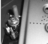
Figure 7. Ignitor assembly beside the burner.
